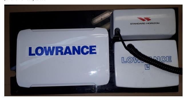
To make things easier in the spring, I wanted to test the connection between the VHF radio and the HDS9. To do this, I needed to power them both up and connect the NMEA 0183 wires. I laid the dash panel on top of a cardboard box and cut matching holes to let the equipment sit down properly. Then I cut a hole in the side of the box to access the wiring.
